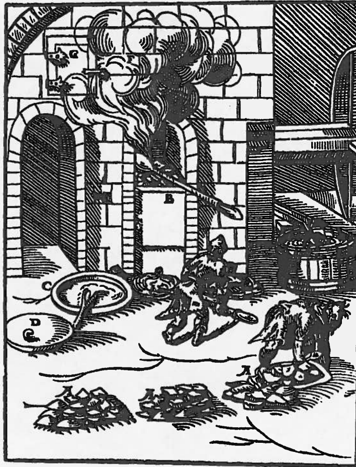
Figure 18. Furnace for the melting of copper and lead as depicted by Lazarus Ercker in 1580.
